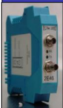
The 2E46 Optical Interface Module connects the EOTec 2000 modem with the fiber cable network allowing the optical signals to be transmitted to and received from another fiber optic modem.
